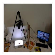
Negatives are scanned with a light box. The light box provides the lighting needed for a clear picture. It projects the light through the negative. Because it's a negative, the image has to be inverted with software.
