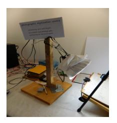
Wooden light stands and clip on utility lights using 60 W. fluorescent bulbs are inexpensive and can be set up quickly.
