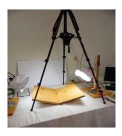
A pair of wooden boards makes a cradle to hold old books and prevent damage to the bindings. The camera must be angled to give a flat view of each page.
